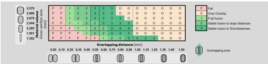
Figure 3. Figure 3: Mapping of the effect of overlapping and material amount. “F” refers to failure to fuse. “O” refers to over-overlapping. 1 - Frail contour fusion. 2 - Stable fusion for long HF. 3 - Stable fusion for short HF, after which it becomes over-overlapping.
